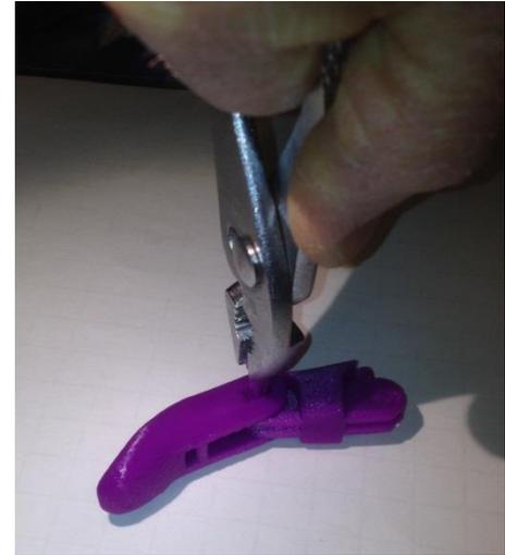
With the rectangular hole on the top align the holes in the thumb tip and thumb proximal phalanges (the wide one).
